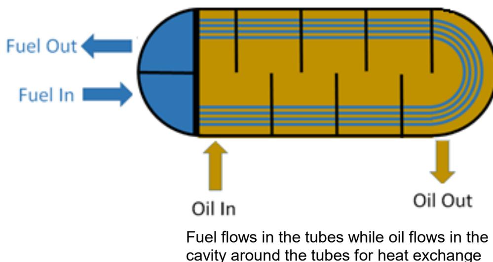
Figure 1: Schematic diagram of MFOHE
