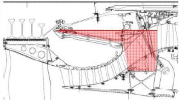
b: Maximum storage capacity of A Sump reached due to fuel leak
