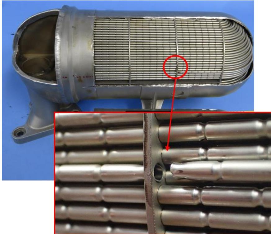
Figure 2: View of cracked tube in MFOHE
