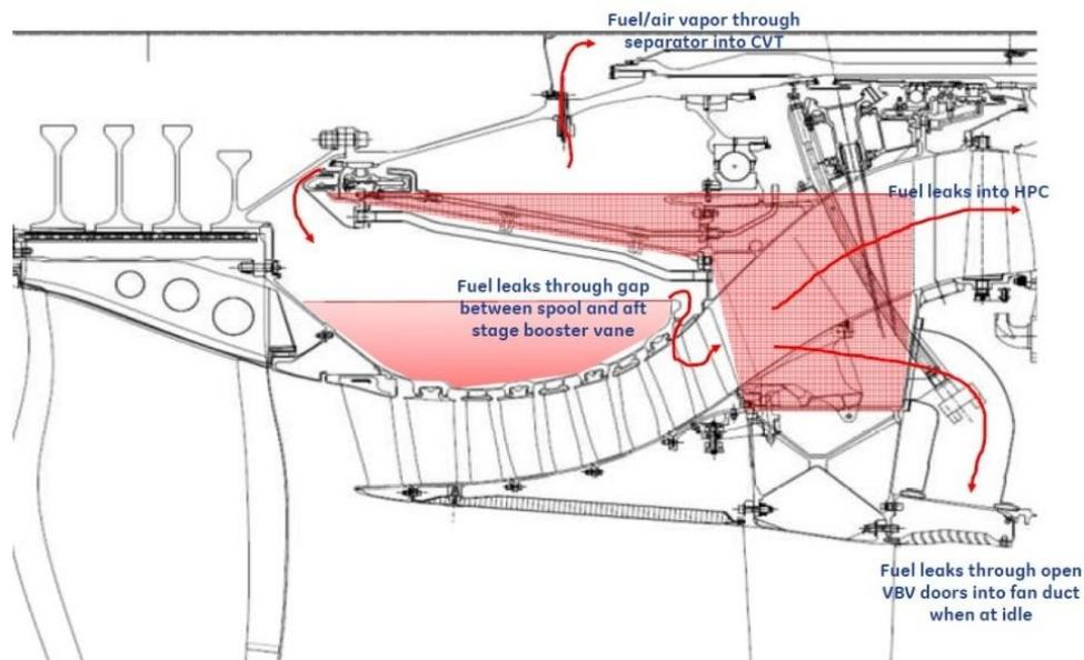
Figure 4: Leak path for fuel
