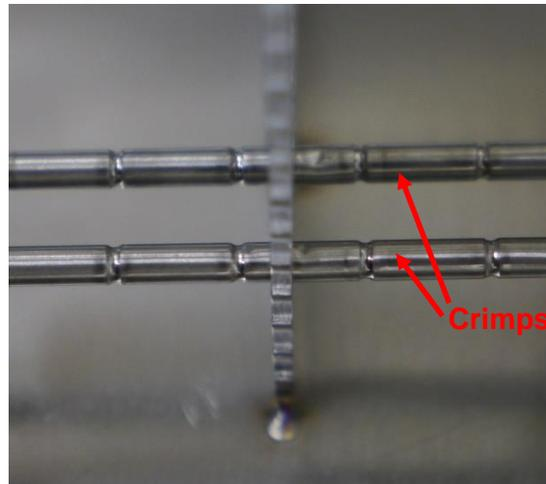
Figure 5: Crimps on tubes
