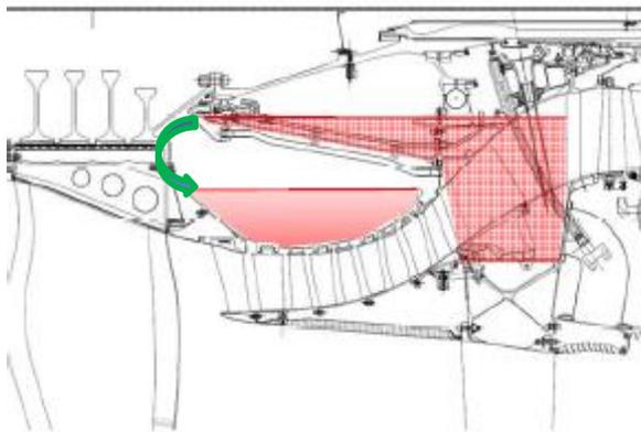
c: Fuel leaked into the booster spool cavity
